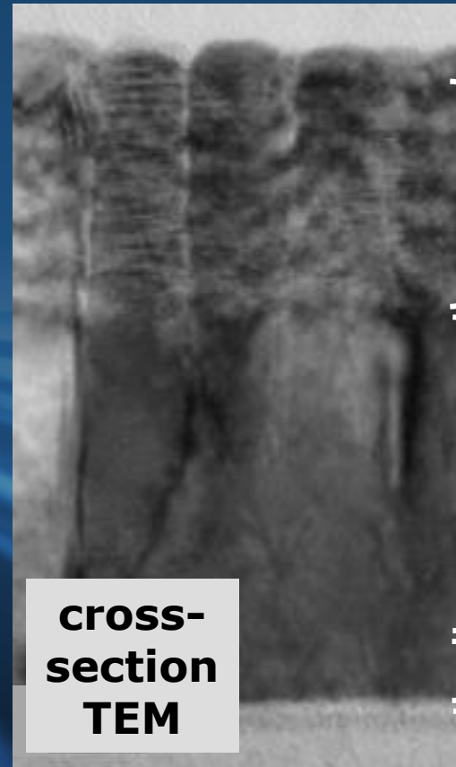
CoCrPt alloy with Oxide segregant
