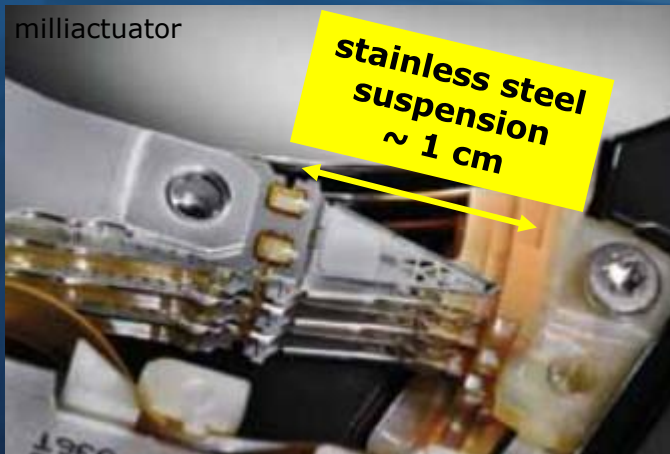
Heads shown parked on loading ramp
