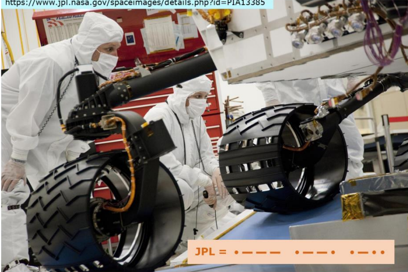
A Wheel Check at NASA's Jet Propulsion Laboratory. Curiosity has six wheels each independently driven ( note JPL in morse-code formed into the wheel tread )
